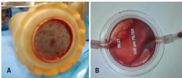
**Figure 2.** (A) Reusable filter. (B) Disposable filter
